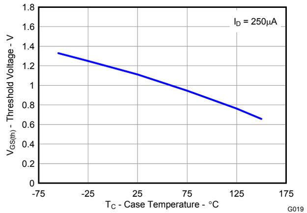
Figure 19. Sync MOSFET V<sub>GS(th)</sub>
