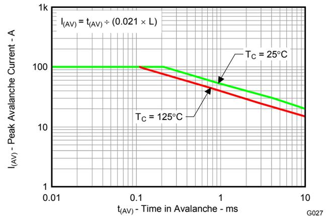
**Figure 27. Sync MOSFET Unclamped Inductive Switching**
