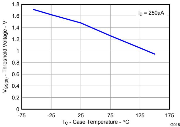
Figure 18. Control MOSFET V<sub>GS(th)</sub>
