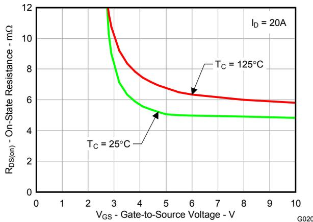
Figure 20. Control MOSFET R<sub>DS(on)</sub> vs V<sub>GS</sub>
