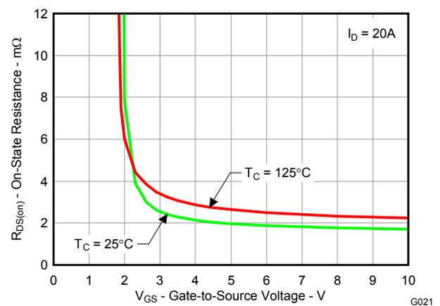
Figure 21. Sync MOSFET R<sub>DS(on)</sub> vs V<sub>GS</sub>
