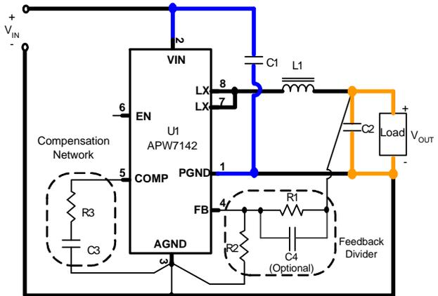
2. In Figure 2, the loops with the same color bold lines conduct high slew rate current. These interconnecting impedances should be minimized by using wide and short printed circuit traces.
