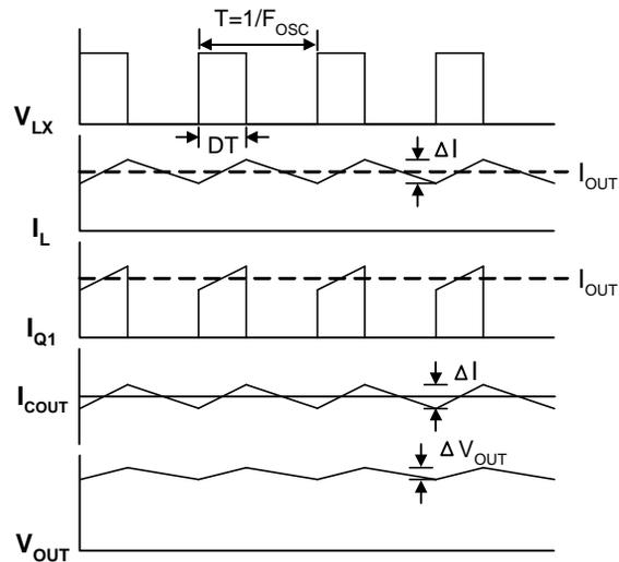
Figure 1 Converter Waveforms
