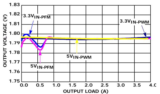
FIGURE 12.  $V_{OUT}$  REGULATION vs LOAD (1MHz,  $V_{OUT} = 1.8\text{V}$ )
