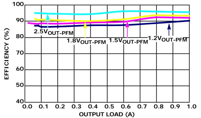
FIGURE 4. EFFICIENCY vs LOAD (1MHz 3.3  $V_{IN}$  PFM)
