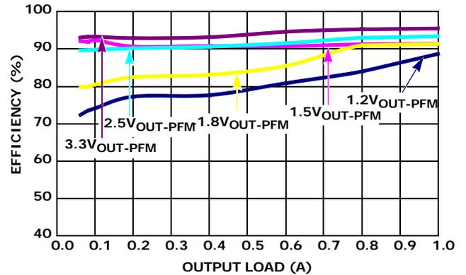
FIGURE 6. EFFICIENCY vs LOAD (1MHz 5 $V_{IN}$  PFM)
