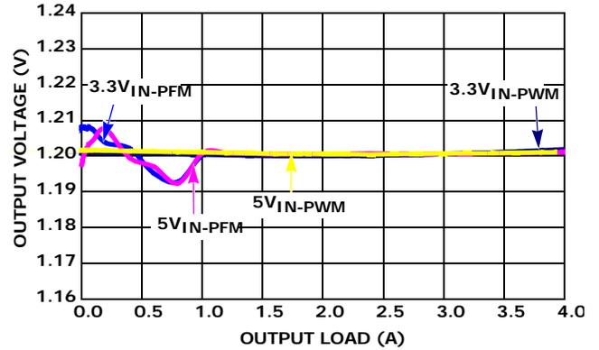
FIGURE 10.  $V_{OUT}$  REGULATION vs LOAD (1MHz,  $V_{OUT} = 1.2\text{V}$ )
