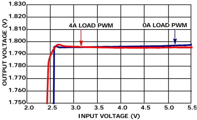
FIGURE 15. OUTPUT VOLTAGE REGULATION vs VIN (PWM  $V_{OUT} = 1.8$ )
