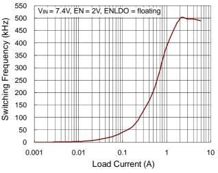
Switching Frequency vs. Load Current
