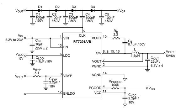
Figure 1. Typical Application Circuit with Pure MLCC Solution
