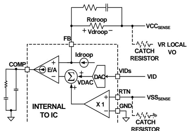
FIGURE 16. DIFFERENTIAL SENSING AND LOAD LINE IMPLEMENTATION
