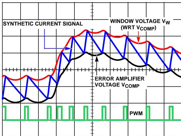
FIGURE 12. MODULATOR WAVEFORMS DURING LOAD TRANSIENT
