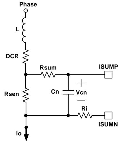
FIGURE 24. RESISTOR CURRENT-SENSING NETWORK
