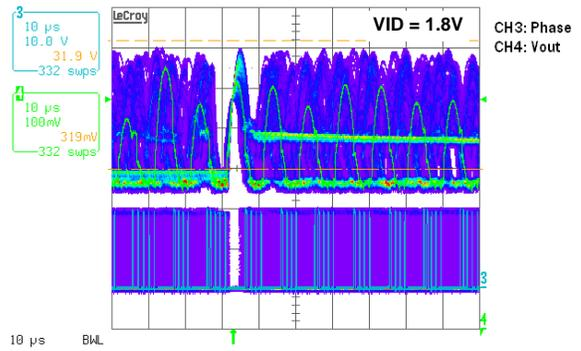
FIGURE 3. PS0, 1-35A HIGH REP LOAD TRANSIENT
