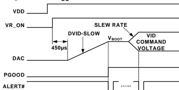
FIGURE 15. SOFT-START WAVEFORMS
