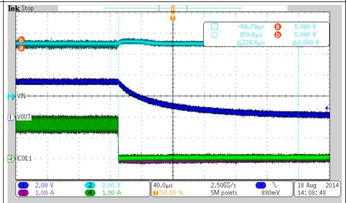
$V_{IN} = 5.0 \text{ V}$  (Falling)
