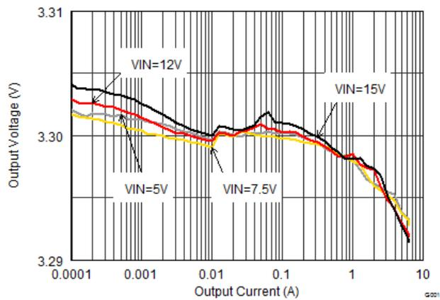
Figure 19. Output Voltage vs Output Current (Load regulation)
