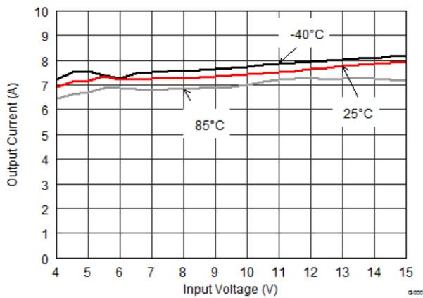
Figure 21. Maximum Output Current vs Input Voltage
