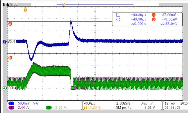
$V_{OUT} = 1.8\text{ V}$        $C_{OUT} = 6\text{x}47\ \mu\text{F}$
