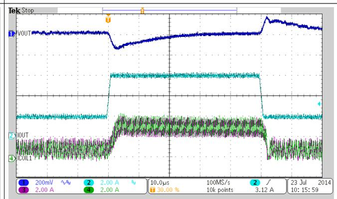
Figure 46. Load Transient Response (PWM-PWM)
