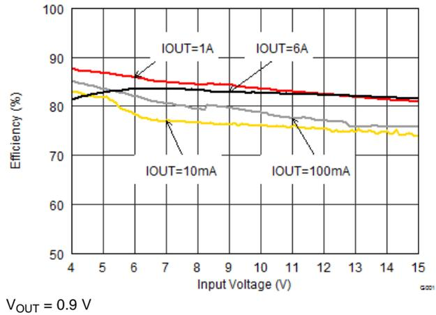
Figure 18. Efficiency vs Input Voltage
