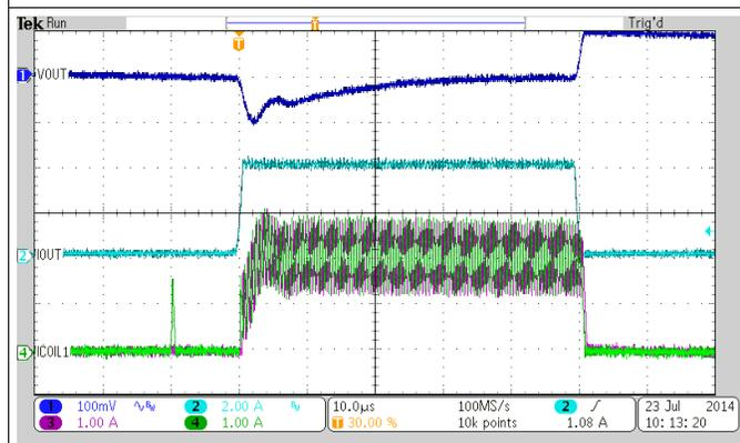
Figure 45. Load Transient Response (PSM-PWM)
