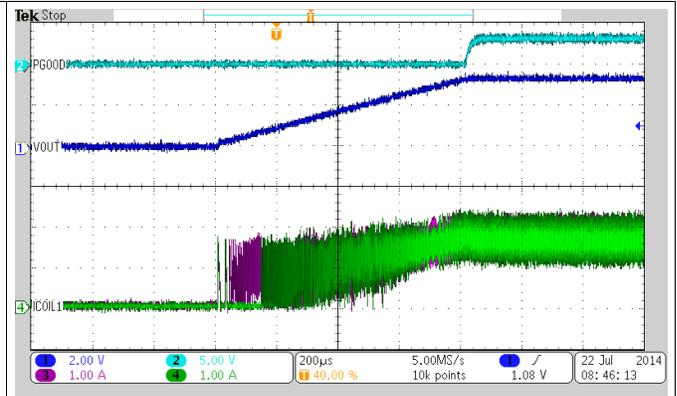
Figure 24. Startup into 1 Ω (3.3 A)
