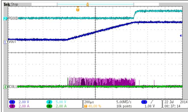
Figure 23. Startup into 33 Ω (100 mA)
