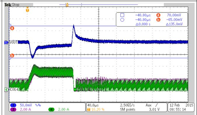
$V_{OUT} = 1.8\text{ V}$        $C_{OUT} = 6\text{x}47\ \mu\text{F}$       additional  $C_{FF} = 82\ \mu\text{F}$
