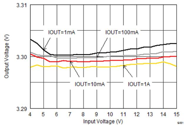
Figure 20. Output Voltage vs Input Voltage (Line regulation)
