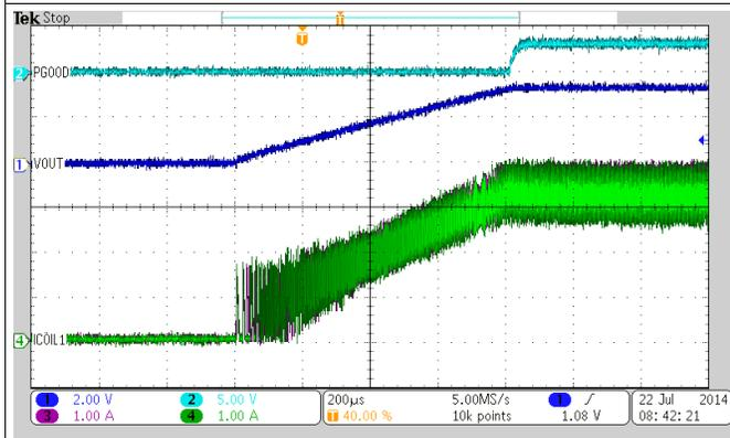
Figure 25. Startup into 0.5 Ω (6.6 A)
