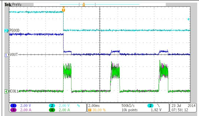
Figure 36. HICCUP at Short Circuit
