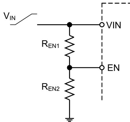
Figure 40. Resistive Divider for Controlled EN Threshold
