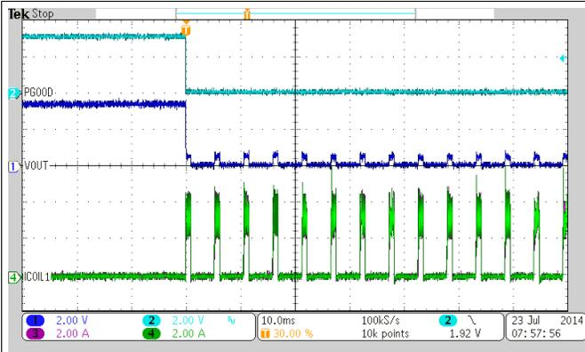
Figure 35. HICCUP at Short Circuit
