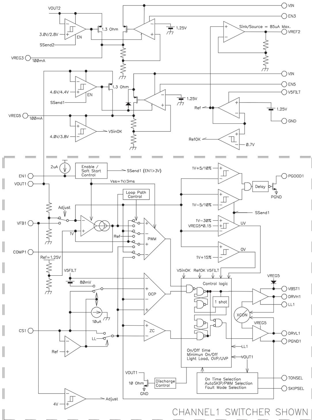
Figure 27. Block Diagram (One Channel Only Shown)
