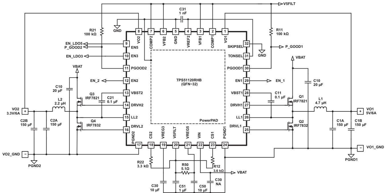
Figure 30. D-Cap Mode, Fixed 5-V / 6-A, 3.3-V/6-A, R<sub>DS(on)</sub> Sensing
